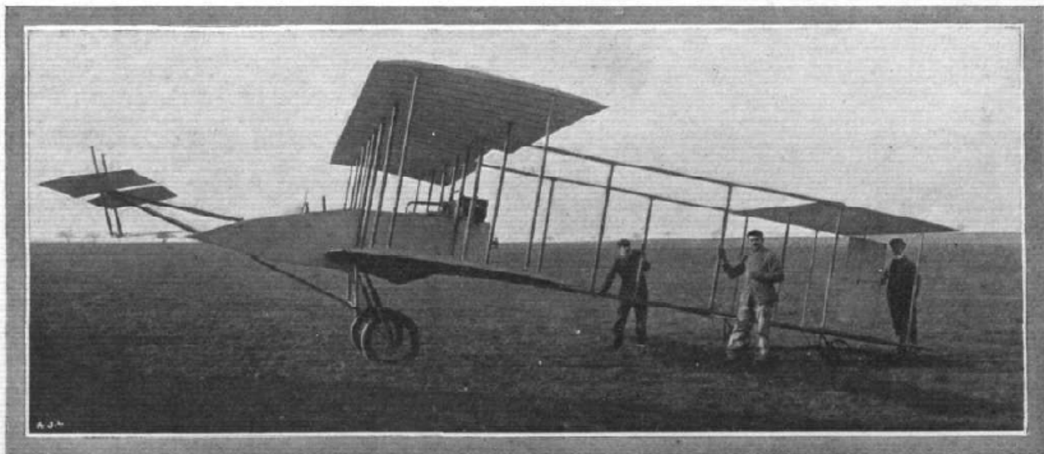
THE MAURICE FARMAN AEROPLANE.—Side view showing the double decks, the elevator in front, and the single rudder between the double-deck tail behind. The spread of the main wings is 10 metres, and the total weight 450 kilogs. The engine at present installed is a 50-60-h.p. Renault. The propeller is not shown.
