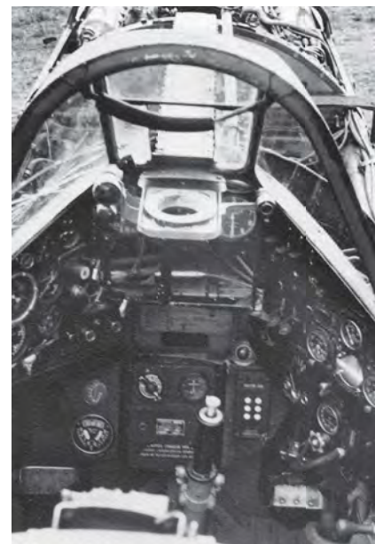
ABOVE: A detailed cockpit view of captured MS406 number 1013, found by German troops at Dreux in June 1940. The Morane fighter had a unique 'wraparound' layout to its instrument panel not seen in other contemporary types.
